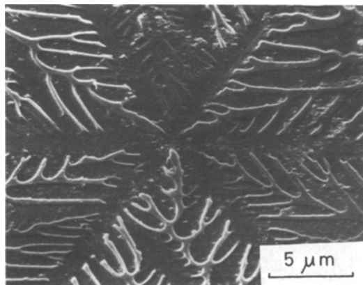
Figure 5 A scanning electron micrograph of a \{111\} surface grown in 70 wt% Fe–30 wt% Ni alloy.
